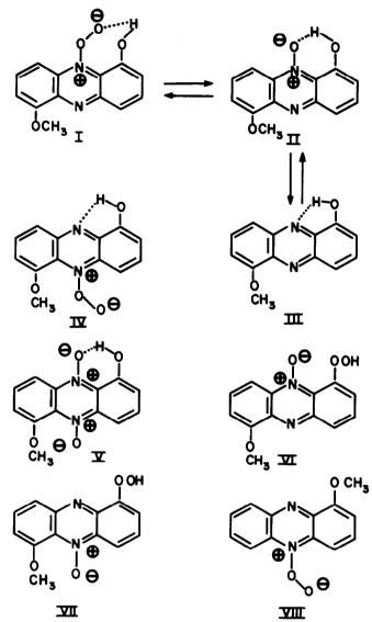
myxin in 71% aqueous 2-propanol at pH 4.76 gave three twoelectron waves at +0.30, -0.102 and -0.308 volts relative to the standard calomel electrode.
